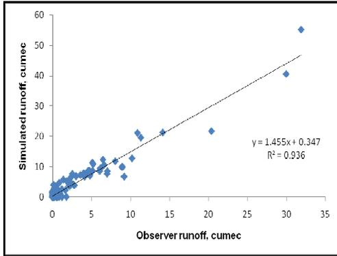
**Fig. 4:** Scatter plot for the observed and simulated monthly surface runoff during calibration period (1998-2007).
