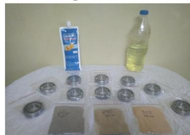
Fig. 2.1: Bearing samples
