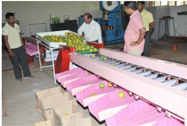
Fig. 3: Testing of Commercial Scale Fruit Grader with Orange
