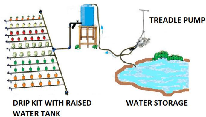
Fig.5: Drip kit with treadle (foot) pump for vegetable garden
