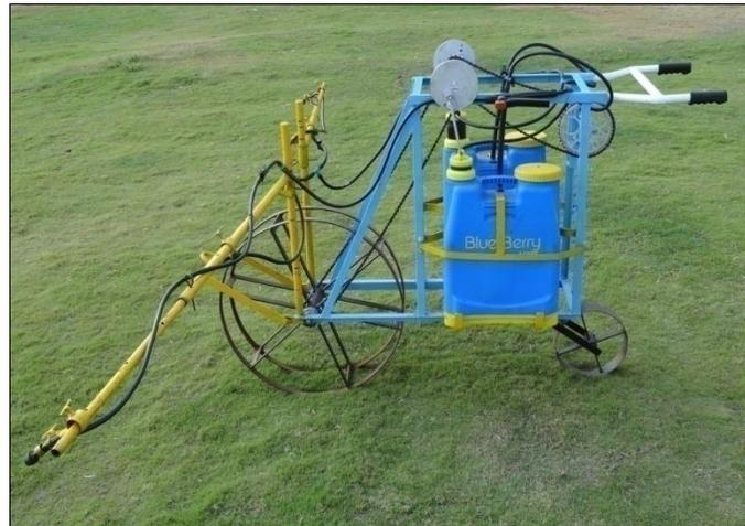
**Fig.1: Manually Operated Wheelbarrow Sprayer**
